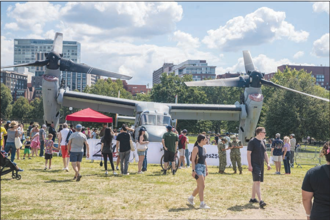
People got to get a closer look at the MV-22B Osprey, an aircraft that takes off and lands vertically but offers the speed and range of a turboprop plane.
