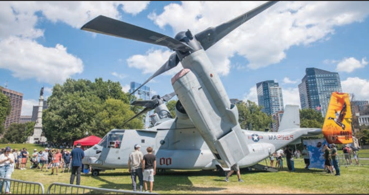
People got to get a closer look at the MV-22B Osprey, an aircraft that takes off and lands vertically but offers the speed and range of a turboprop plane.
