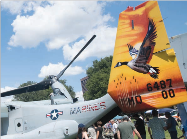
People got to get a closer look at the MV-22B Osprey, an aircraft that takes off and lands vertically but offers the speed and range of a turboprop plane.
