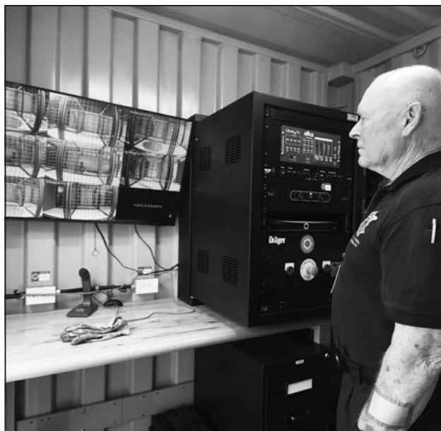
Advanced Fire Skills Program Coordinator Al Beardsley stands in the new SCBA Maze Trailer’s control room, which features a digital audio and video feed from multiple cameras inside the training area. Instructors can communicate with trainees and control lights and sound at all times.
